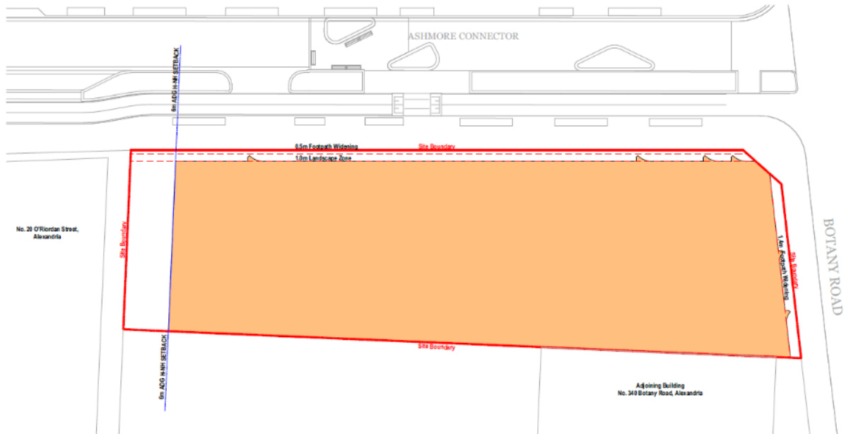
Figure 3: Proposed envelope plans - Levels 4 - 7 (Note: proposed blade projections above ground level over setbacks)
